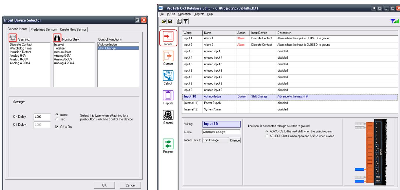
By default, the input (either the + or – terminals) should be grounded using a switch of some kind (toggle, push-button, relay, etc.). The shift will advance when the input detects that it is open. Any subsequent shift advances requires that the input be grounded and then opened again. To identify what shift is currently being used, the input 10 LED on the top of the Cv3 will be off for shift 1, solid green for shift 2, flashing green for shift 3 and flashing orange for shift 4.
