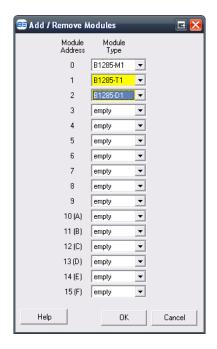
The modules are assembled and shipped with the physical addresses to match (ie: the M1 module is always address 0, the callout module is always address 1 and the expander modules are always 2 and above – from bottom to top).
