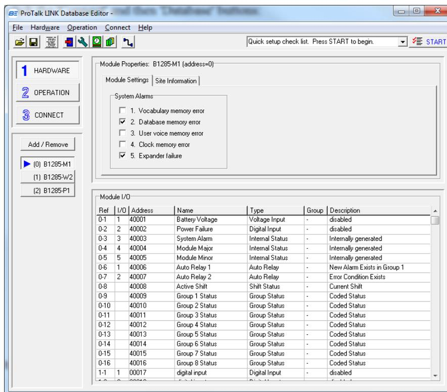
Press the 'Add/Remove' button and then change the W2 to a W3 from the drop-down-box:
