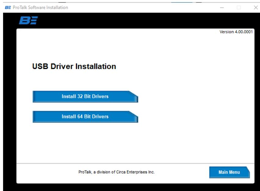
Select either the 32-bit or 64-bit drivers. Most modern PCs have the 64-bit version of Windows, though if you're not sure what version you have, open the Control Panel and check:
